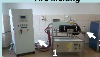
Linn MFG-30 induction furnace: 1 – voltage generator; 2 – melting induction furnace.
