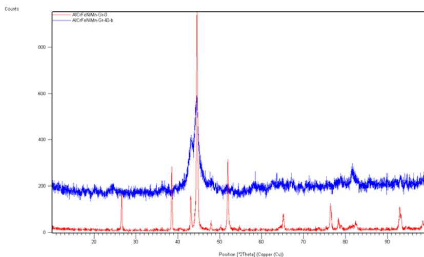
Figure 3. XRD patterns at 0 and 40 h milling time of AlCrFeMnNiGr HEA composite.
